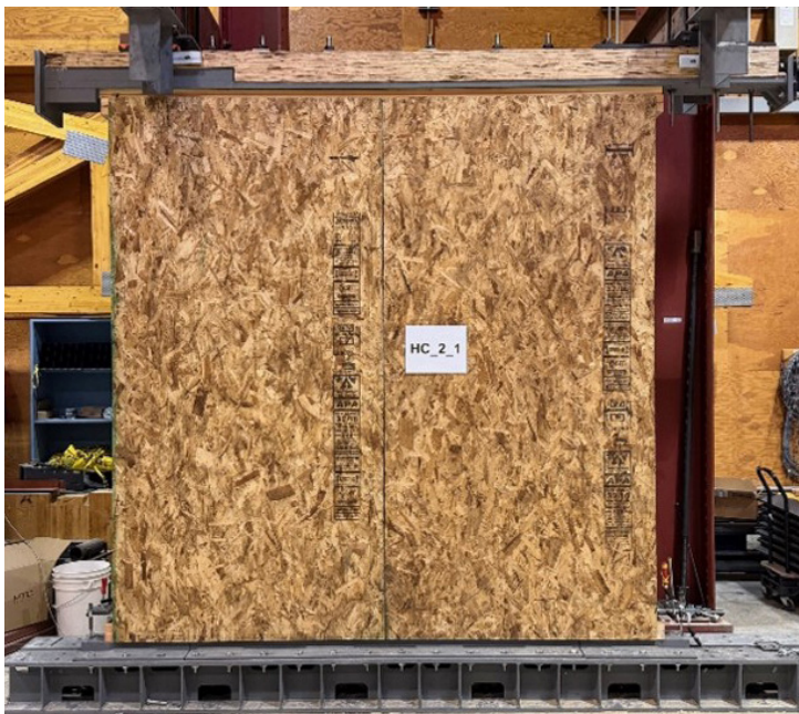
Full-scale experimental test on a high-capacity shear wall
