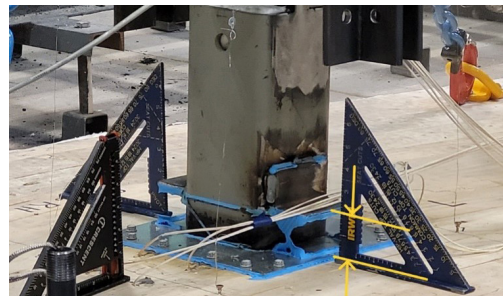
Test 1: Upward differential displacement of the MPSC during fire testing.
