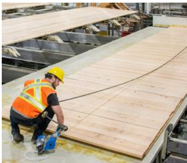
(left) Mass timber panels prefabrication | Photo credit: Matthew Bolt Photography
