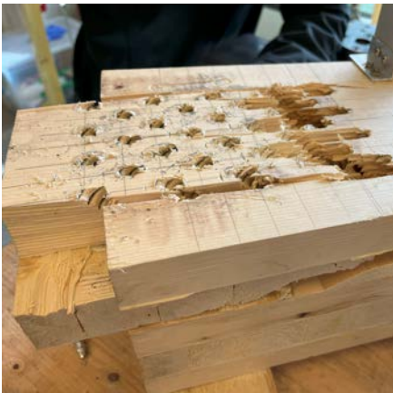
Figure 2: Plug-step shear failure (plug shear in parallel to major strength layers and step shear in perpendicular to major strength layers)
