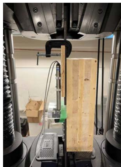
Figure 1: Test set-up of CLT-steel STS connections
