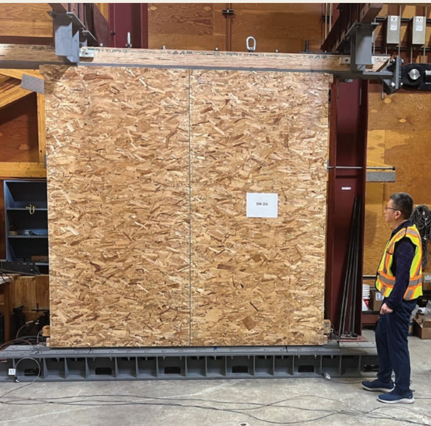
Research into design values for high-capacity shear walls with multiple rows of nails | Photo: FPIInnovations
