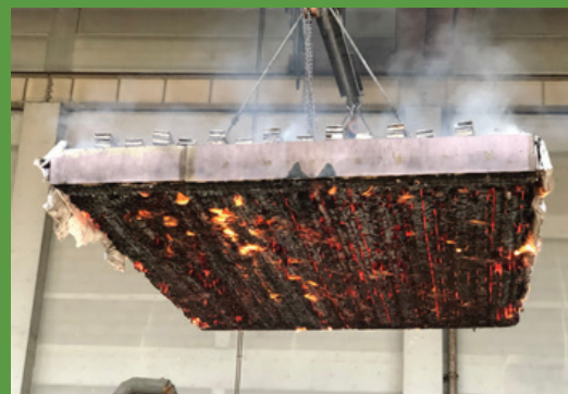
NLT Fire Resistance Test, Beijing / Photo: Canada Wood China
