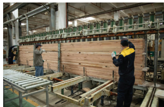
Glulam manufacturing for Wuxi Inspur Big Data Innovation Centre / Photo: Canada Wood China
