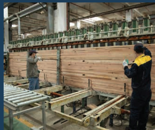
Glulam manufacturing for Wuxi Inspur Big Data Innovation Centre | Photo: Canada Wood China
