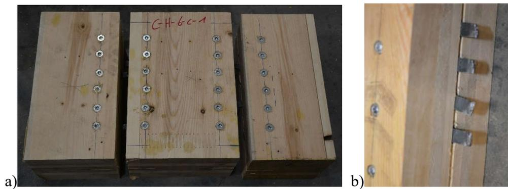
Figure 24: a) Typical test specimen for cyclic IPSP shear connection tests; b) ruptured steel bridges
