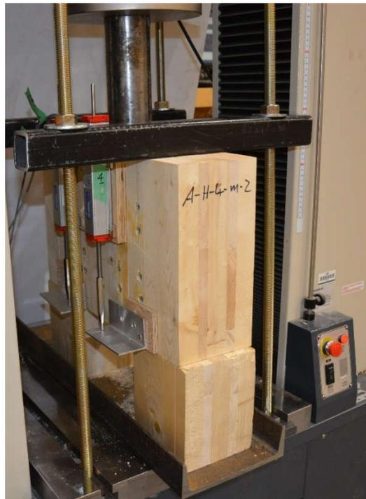
*Figure 10: Test setup for quasi-static monotonic tests*
