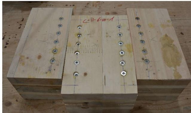
Figure 23: Typical test specimen for monotonic IPSP shear-connection tests
