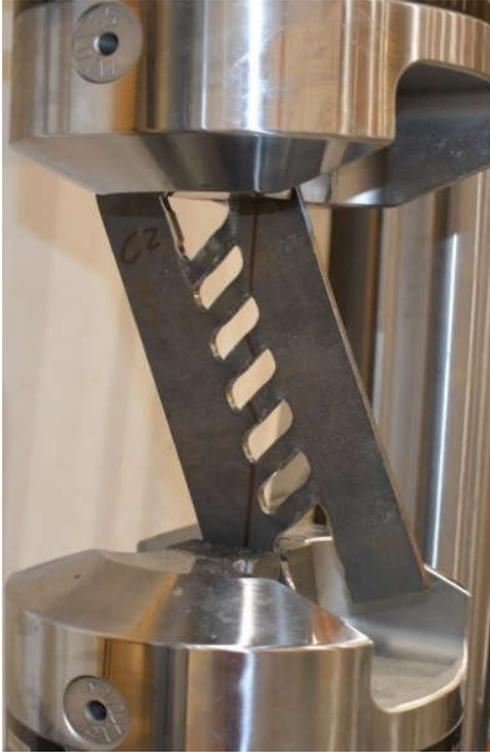
Figure 6: Setup shear-tension test
