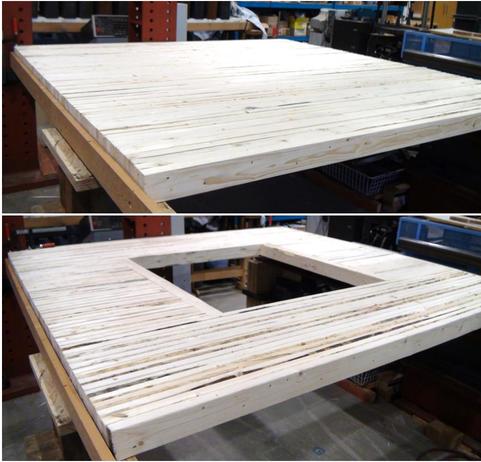
Figure 2 Nail laminated shear wall specimens
