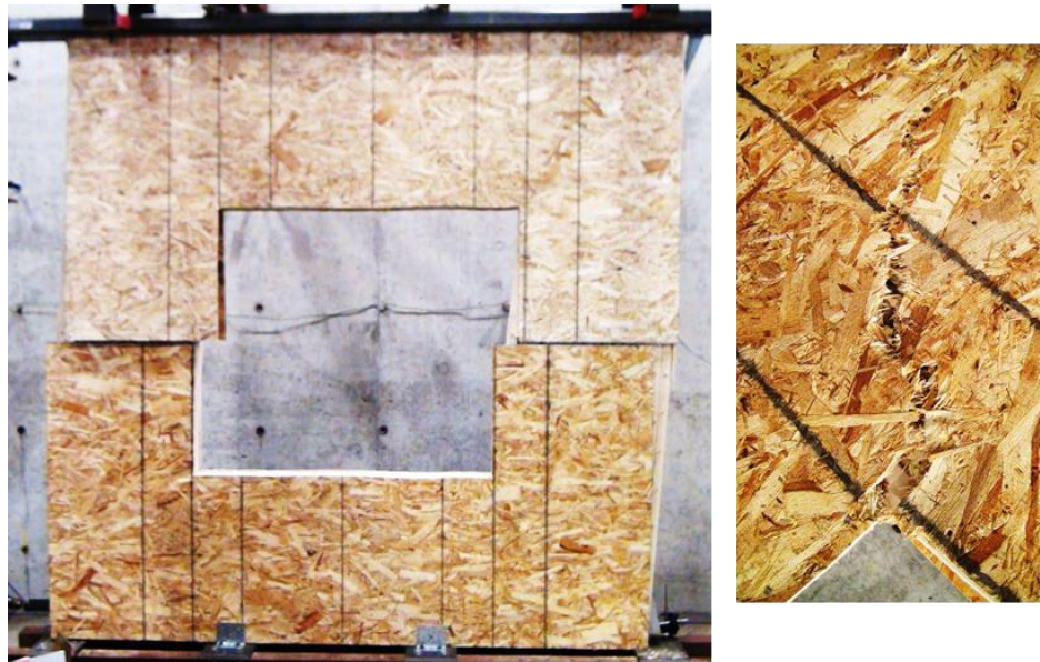
Figure 8 Failure of Wall-F with opening
