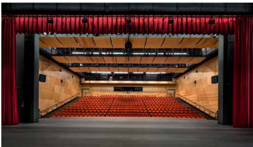
Figure 32. Southern Okanagan Secondary School Venebles Theatre (School District 53) Oliver, British Columbia—Wood Panels Used Throughout Performance Theatre for Acoustic Finish
