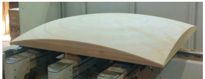
Figure 28. Rendering of the final Positive Mold / Process Photo of the CNC'd Positive Mold
