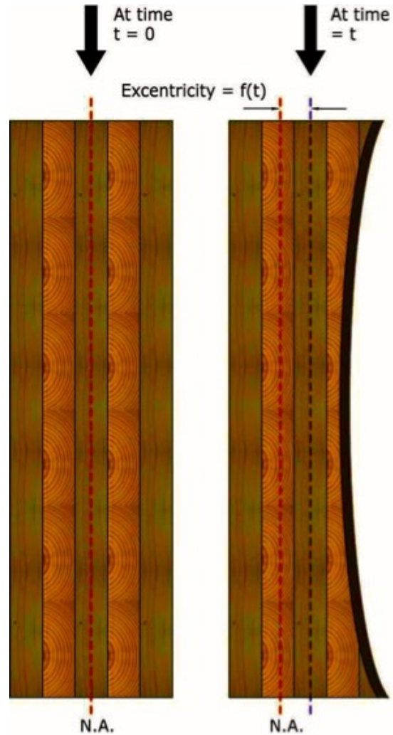
FIGURE 7: SHIFT OF NEUTRAL AXIS IN A HEAVY TIMBER ASSEMBLY DUE TO UNEVEN BURNING (DAGENAIS 2014)
