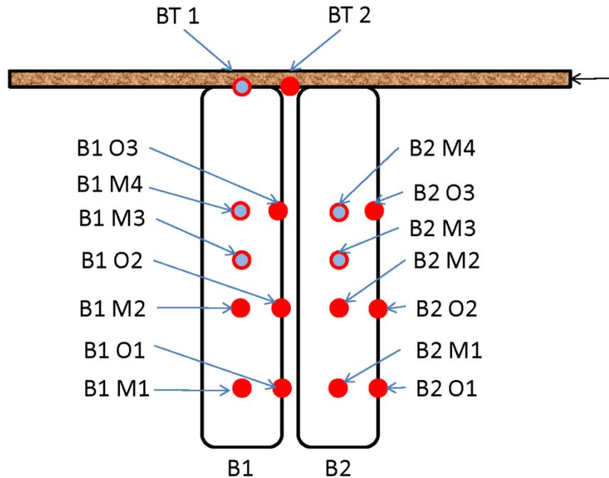
**Figure 4: Location B Interior Thermocouple Locations**
