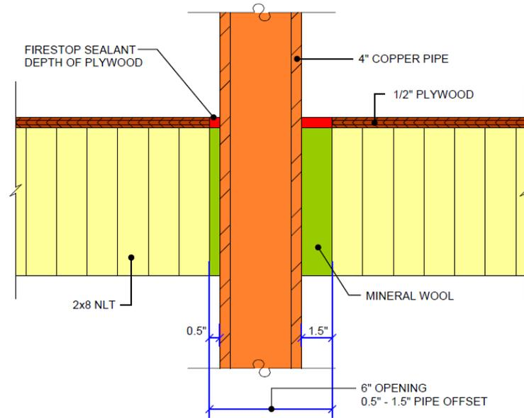
Figure 9. Penetration through NLT. Prepared by GHL Consultants Ltd.
