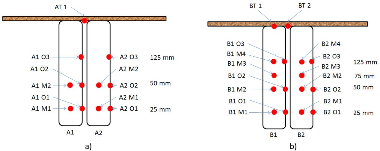
Figure 8. Thermocouple installation locations for Test 2.
