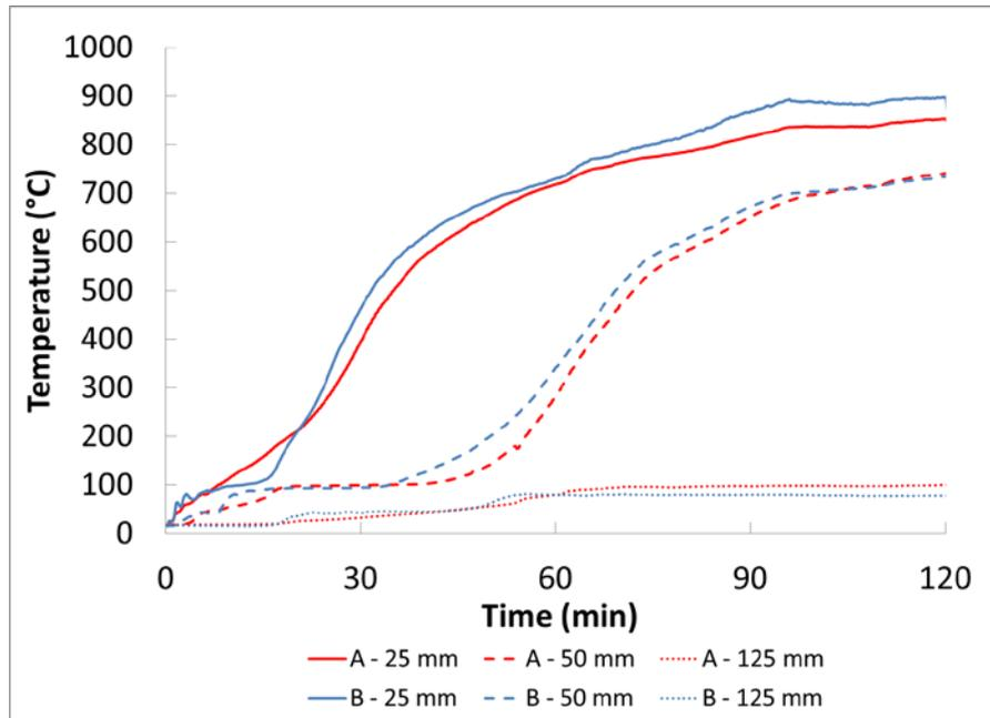
Figure 17. Temperature measurements in spaces between boards
