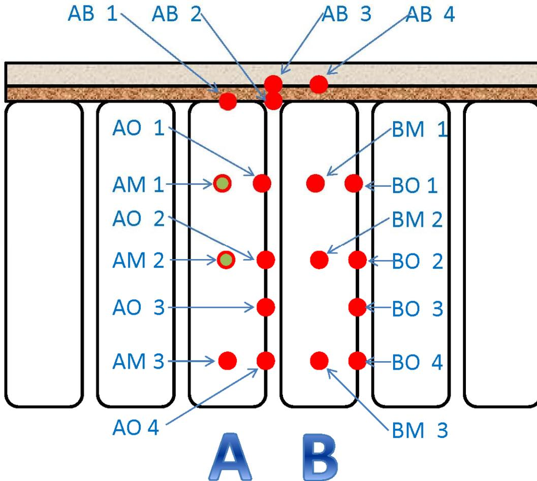
**Figure 3:** Unexposed Thermocouple Locations
