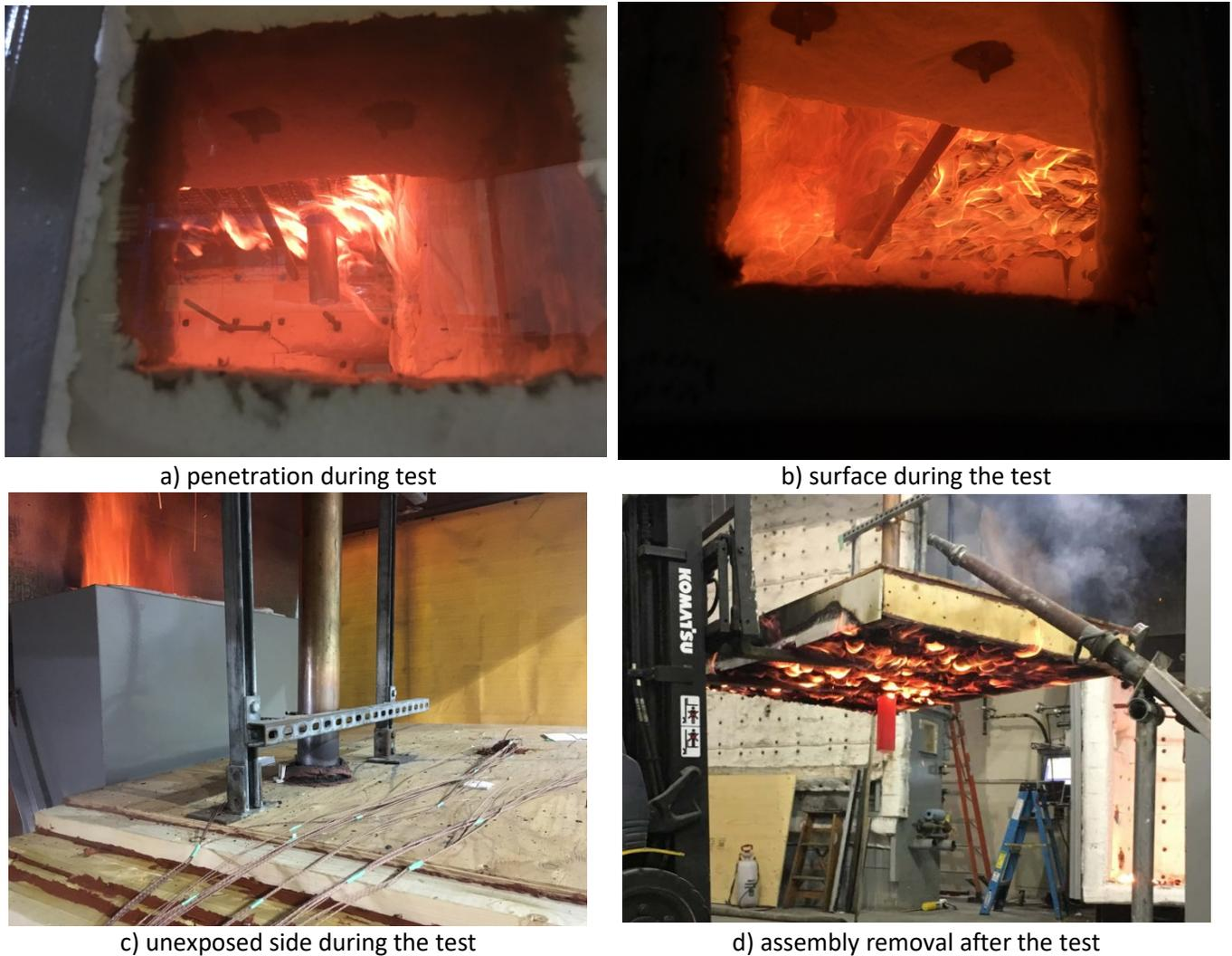
Figure 15. Test 2 assembly during test
