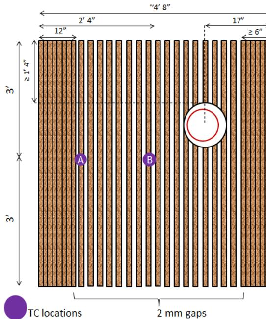
Figure 6. Layout of Test 2. 2x8 NLT with penetration
