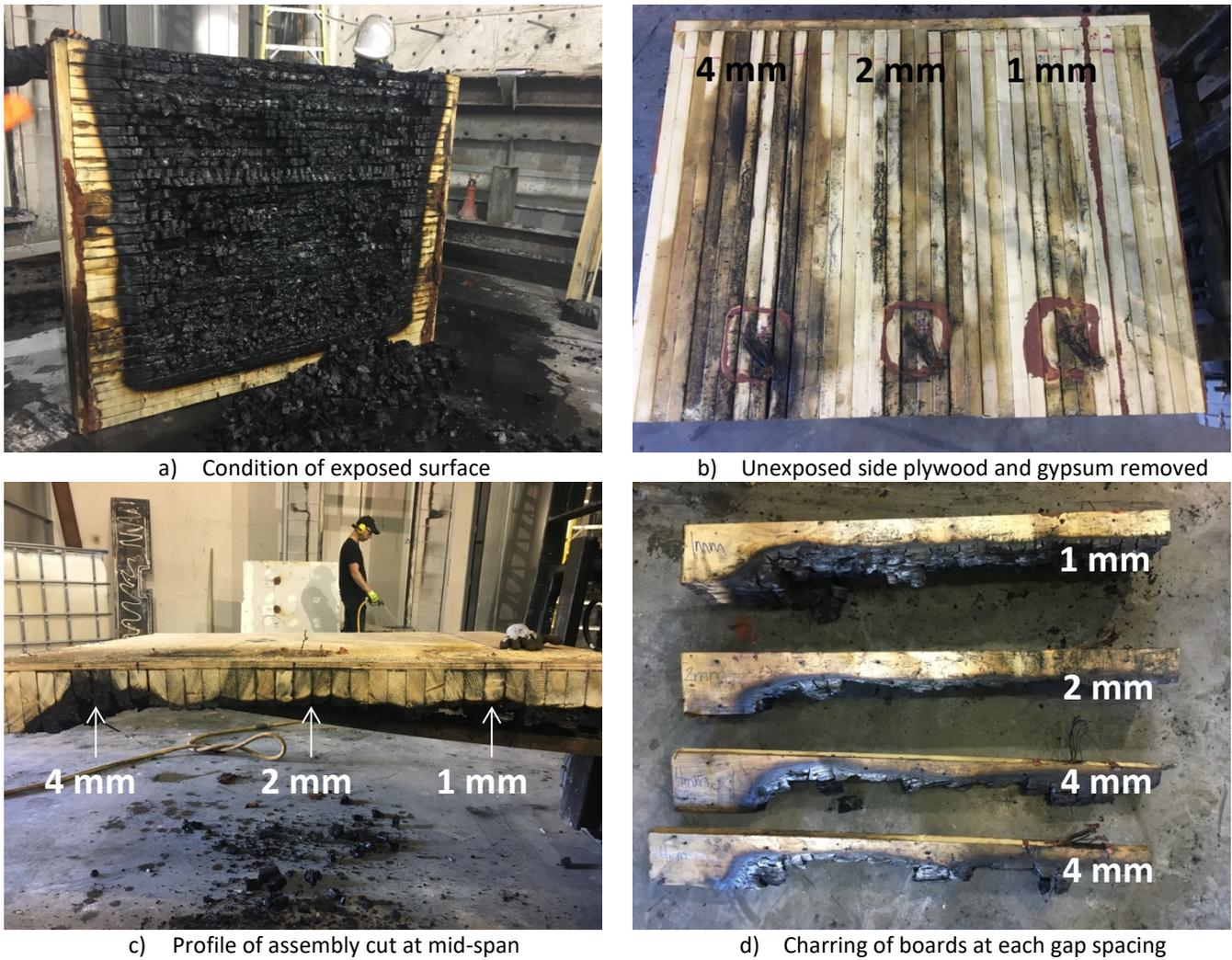
Figure 14. NLT assembly after the test
