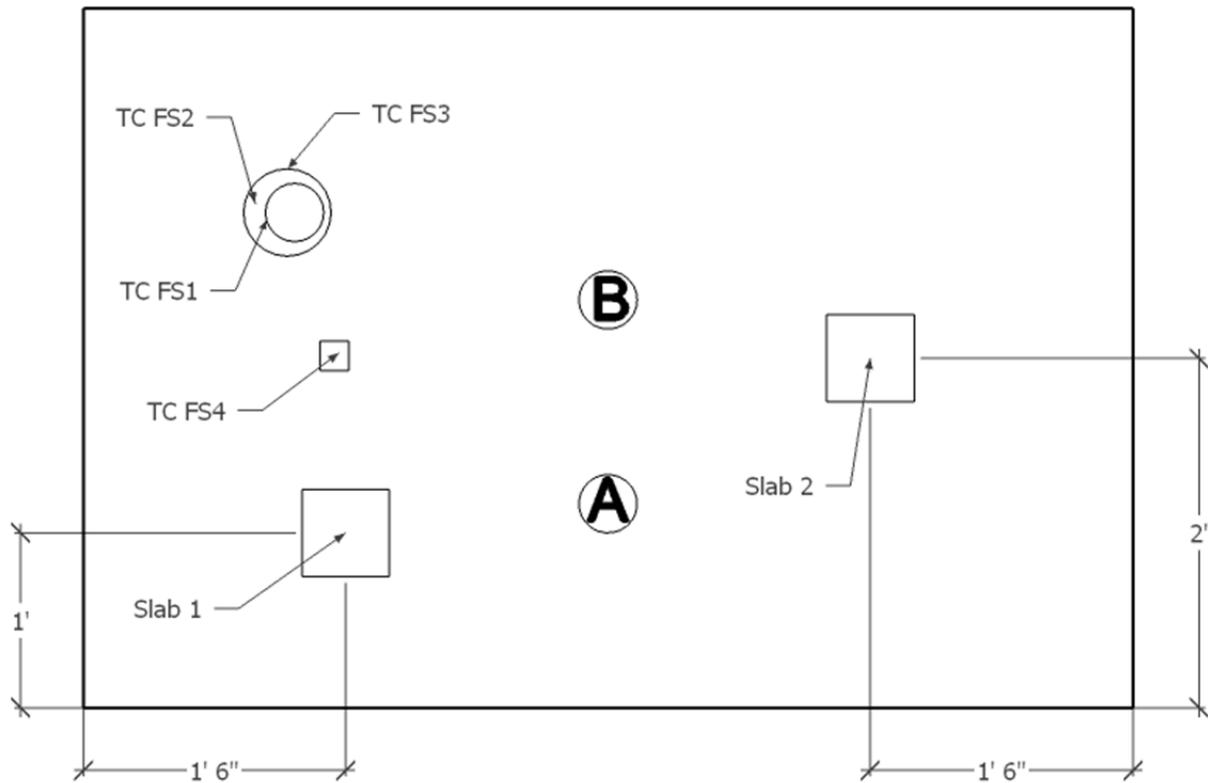
**Figure 5: Unexposed Thermocouple Layout**
