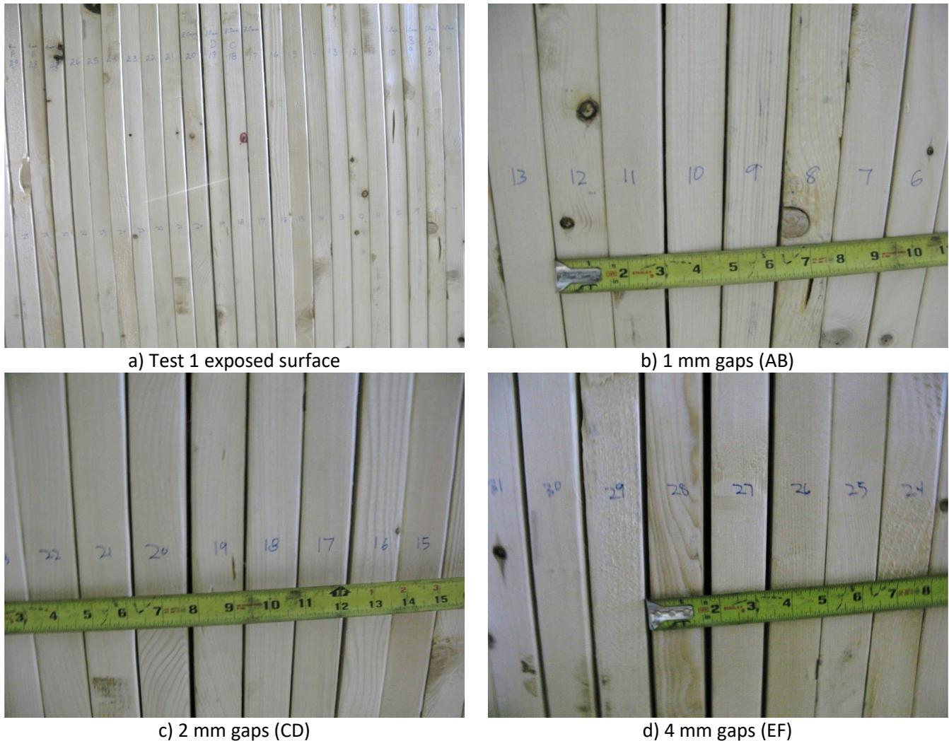
Figure 4. Gap spacing in Test 1
