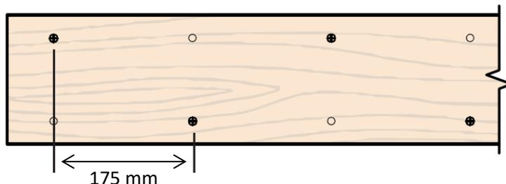
Figure 1. Example of nailing pattern [1]
