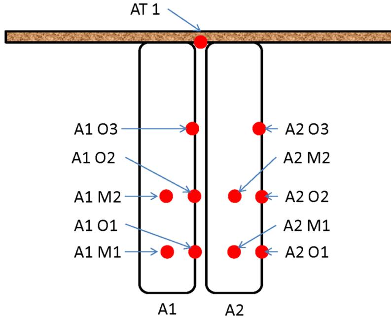
**Figure 3: Location A Interior Thermocouple Locations**
