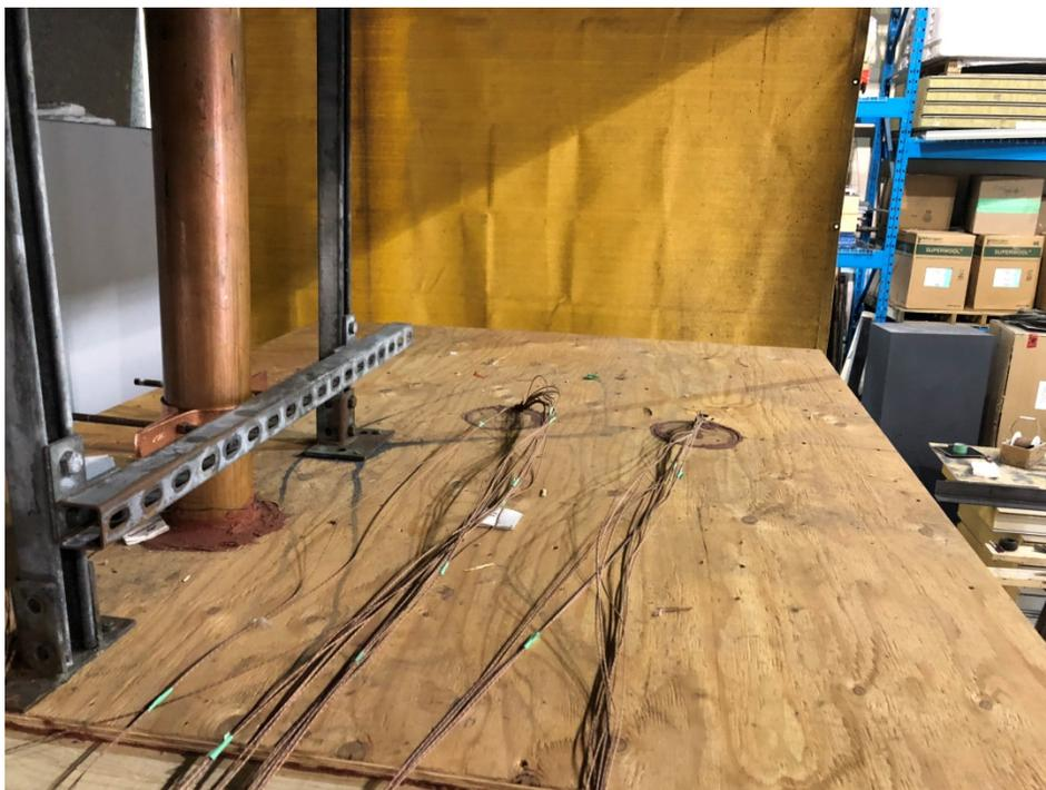
**Figure 10:** The exposed side of the assembly prior to the fire test.
