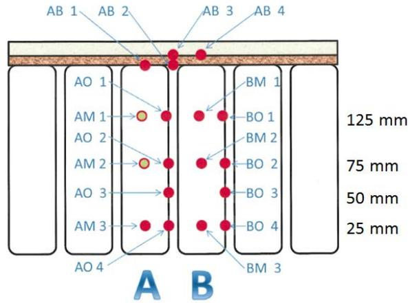
Figure 5. Thermocouple layout for Test 1
