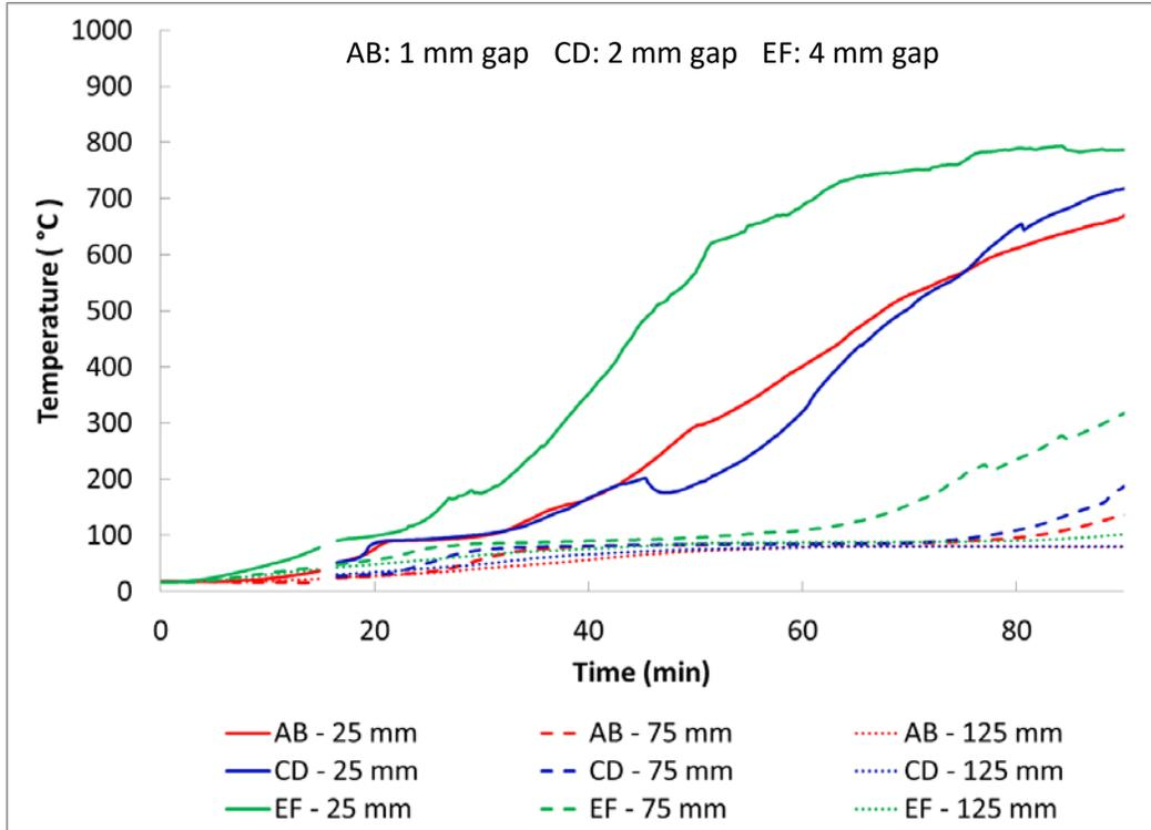
Figure 12. Test 1. Temperature measurements within wood members
