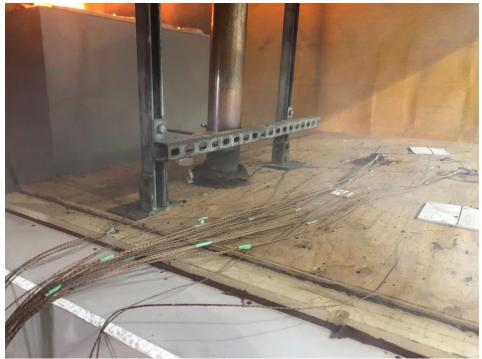
Figure 11: The unexposed side of the assembly at the end of the fire test.
