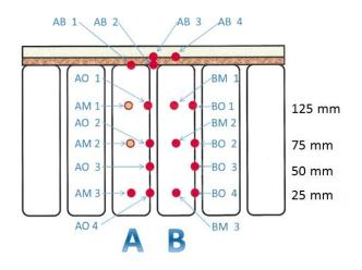
Figure 5. Thermocouple layout for Test 1
