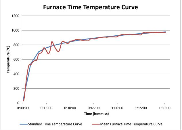
Figure 2: Time Temperature Curve
