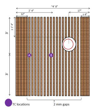
Figure 6. Layout of Test 2. 2x8 NLT with penetration
