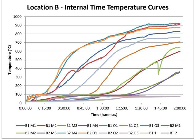
Figure 8: Internal Time Temperature Curves
