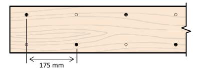
Figure 1. Example of nailing pattern [1]
