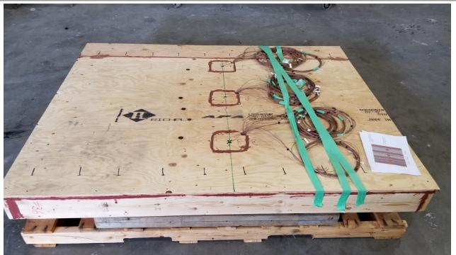
Figure 9: The unexposed side of the assembly prior to the gypsum being installed.
