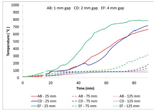
Figure 12. Test 1. Temperature measurements within wood members
