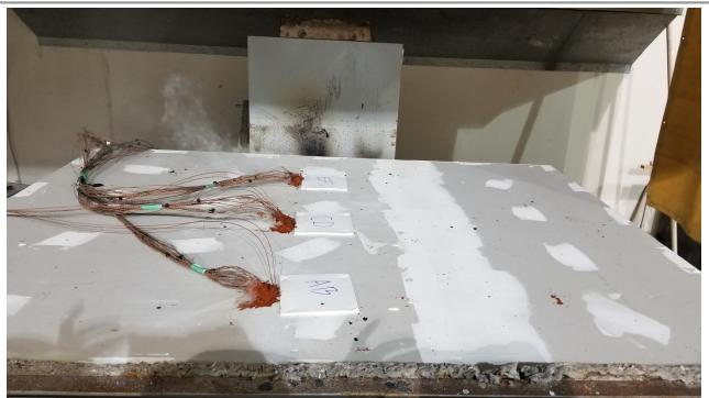
Figure 11: The unexposed side of the assembly during the fire test.
