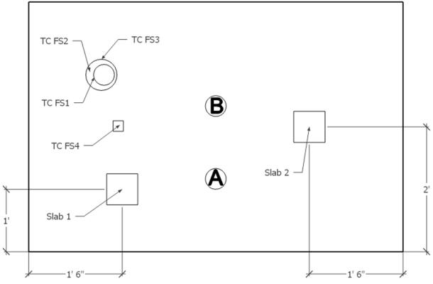
Figure 5: Unexposed Thermocouple Layout
