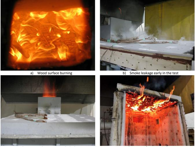
c) Later in the test no smoke leakage
