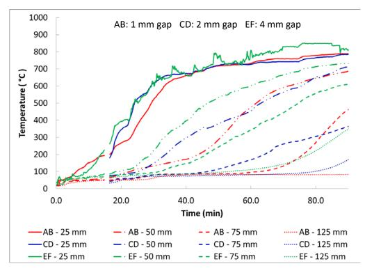
Figure 13. Test 1. Temperature measurements within gaps
