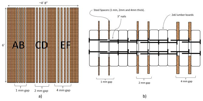
Figure 2. Layout of gap spacing for Test 1. 2x6 NLT
