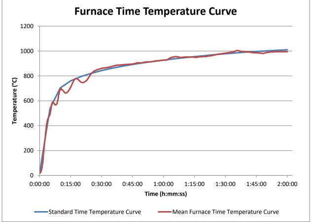
Figure 2: Time Temperature Curve
