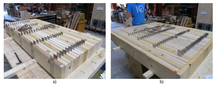
Figure 7. Construction on Test 2 assembly. Installation of spacers
