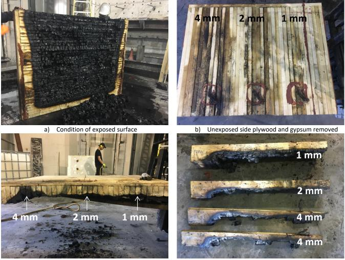
c) Profile of assembly cut at mid-span
