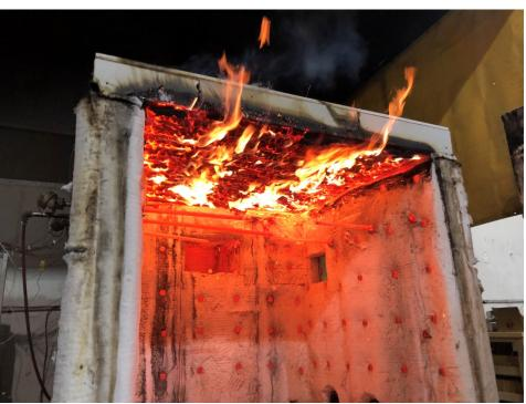
Figure 12: The exposed side of the assembly after the fire test.
