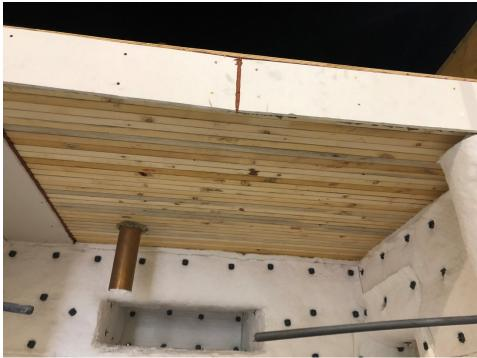
Figure 9: The unexposed side of the assembly prior to the gypsum being installed.
