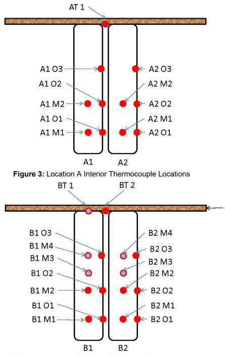
Figure 4: Location B Interior Thermocouple Locations
