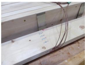
b) installation of thermocouples on outside of boards
