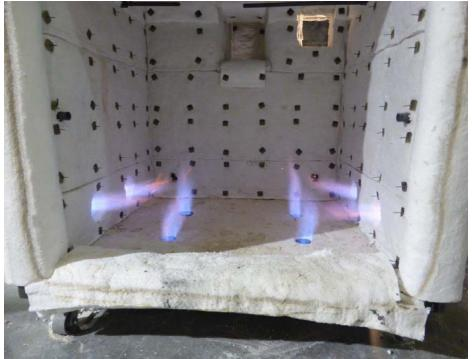
Figure 1: Burners Fired in the Furnace
