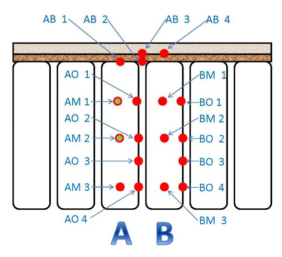
Figure 3: Unexposed Thermocouple Locations
