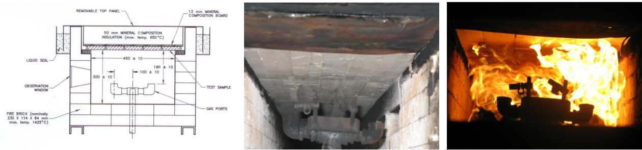
Figure 4 Typical cross-section of the Tunnel test at B-B of Figure 3
